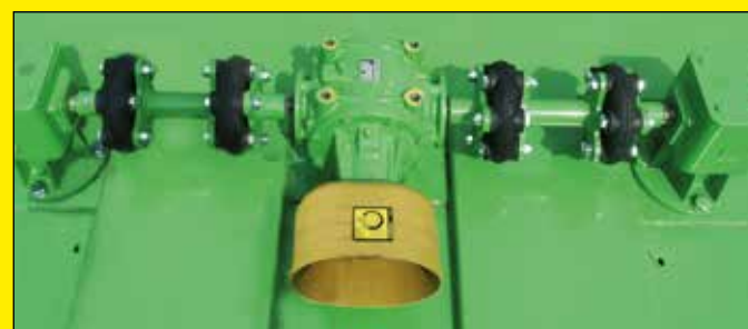
Transmission with four rubber couplings
