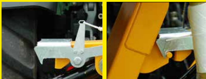
For safety reasons when driving, a mechanical lock prevents the arms from opening
