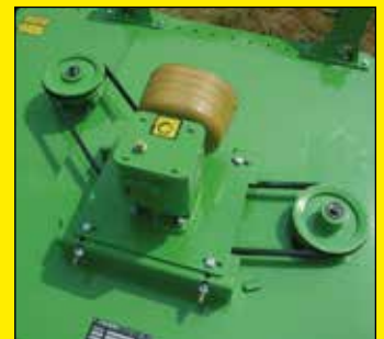
The different rotors are driven by 2 V-belts
