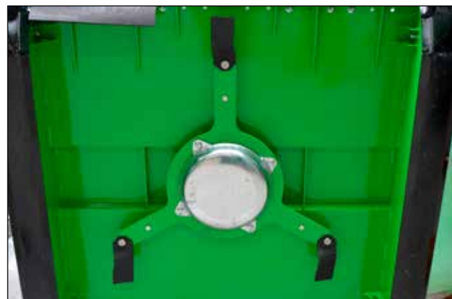
BEV choppers are fitted with a rotor with 3 blades of the "TD type"
