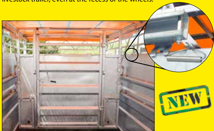
Inner door equipped with handle for a safe opening from the outside
