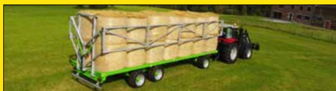
As an option on models 8000D13, 10000T15 and 10000T20, side hydraulic ladders (2 SA) ensure use safety and rapidity
