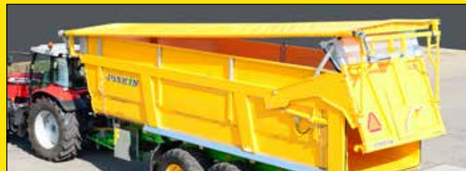
TELECOVER cover compatible with the hydraulic extensions
